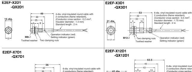
(Conductors (finallie retailed in), (Conductor cross section : 0.5 mm², Insulator diameter : 1.75 mm) Standard length : 2 m
